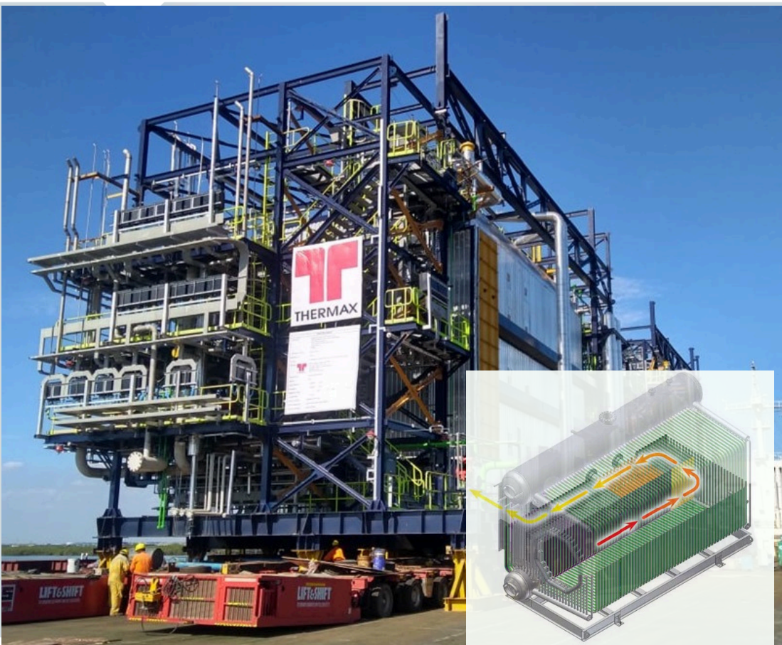
4 units of 400 TPH, 107 kg/cm 2 (g), 520°C Natural Gas fired D-type boiler
